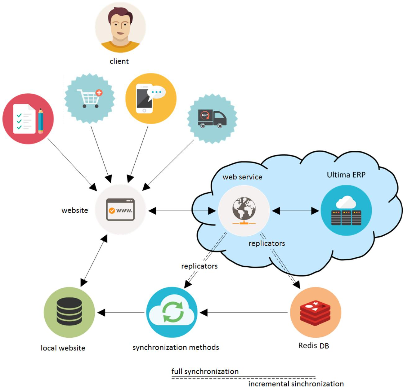
From the provided diagram of interaction it is visible that the website has no access to the database of the company, and all interaction is carried out only through [web service](#).
