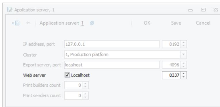
Web developer can receive a list of the available methods of web service to its address <http://localhost:8337/metadata>:
