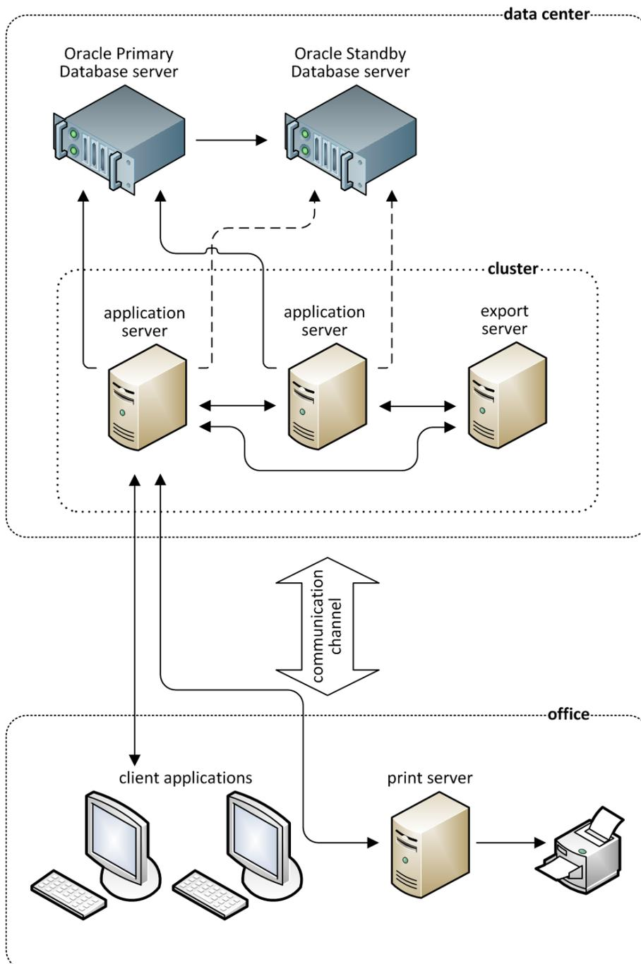
As a rule, and that is highly recommended to, the **database server** is located in the data center. To increase hardware fault tolerance and mitigate the risk of data loss, as well as to share the load, it is recommended to install a standby server/server cluster.
